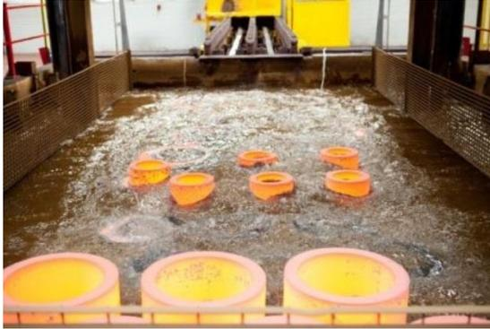
Once the quench has been performed and the material is at ambient, it is in its fully hardened condition. This condition is generally when the material is at or near its highest tensile properties but will be brittle, therefore most hardening operations are performed with a tempering cycle to achieve the required mechanical properties the customer/specification desires.
